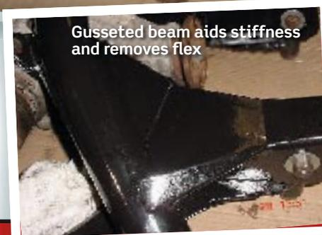
Gusseted beam aids stiffness and removes flex
