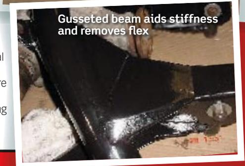
Gusseted beam aids stiffness and removes flex
