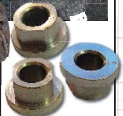
Bobbins allow the floating discs to move a few mm
