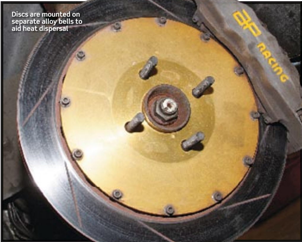
Bobbins allow the floating discs to move a few mm
