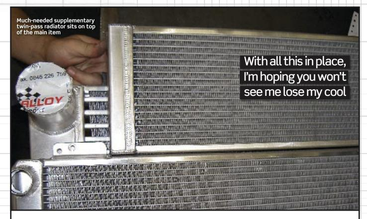
it's side, with the inlet and outlet both at one end. With this supplementary radiator in place, temperatures took a dramatic drop and it was now impossible to exceed 110°C, no matter what the weather.
