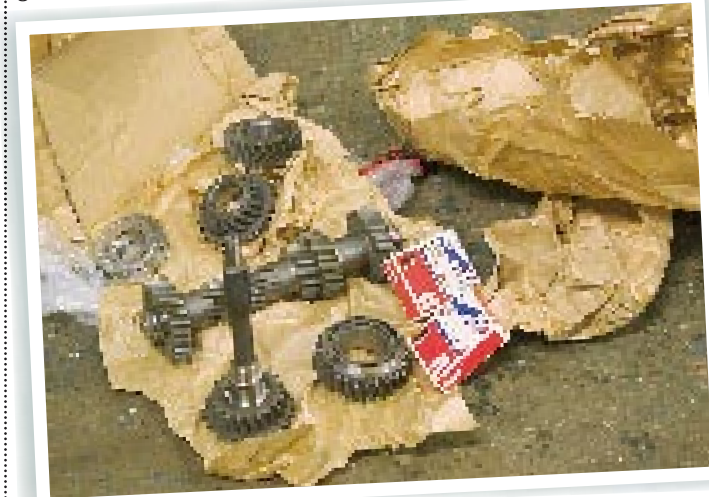
Swedish-made Fixit gearkit features semi-helical, close-ratio gears. Made from quality steel, they're strong, too
